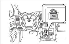
By inserting a mini plug into the AUX audio jack, you can listen to music from a portable audio device through the vehicle's speaker system while in AUX mode.
